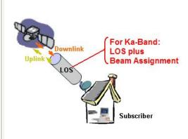
Line of sight (LOS) settings for both Ku-Band and KA-Band include four characteristics: the Azimuth, Elevation, Polarization, and Skew. In Ka-Band transmissions, combining a fifth characteristic, the Beam Assignment, makes data transmission possible.
