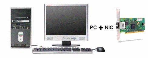
For a computer, or **Internet Ready Device (IRD)**, to have access to a network it will need a **Network Interface Card (NIC)**. This card supplies the <u>physical</u> connection and contains a hardware-embedded **Medium Access Control (MAC) Address**.
