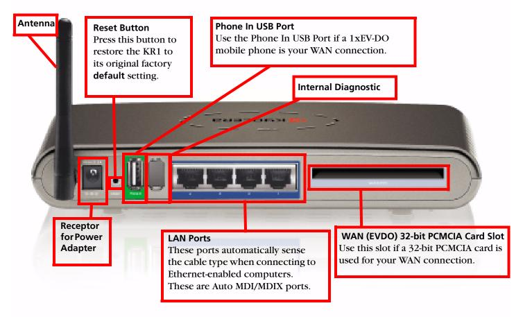
**Note:** The Kyocera KR1 Mobile Router contains two ports: a "Phone-In" USB Port, and a second internal diagnostic port. Please use *only* the "Phone In" USB port for your 1xEV-DO WAN connections. *The second port is not for customer use. Please do not attempt to use this port.*
