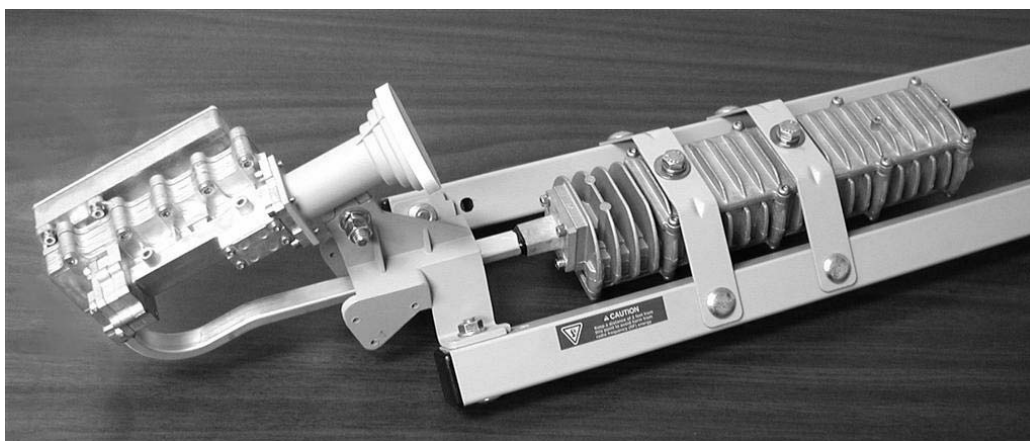
Figure 18: Radio assembly attached to feed arm
