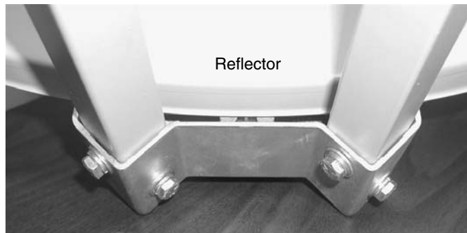
Figure 20: Attaching the feed arm to the reflector bracket
