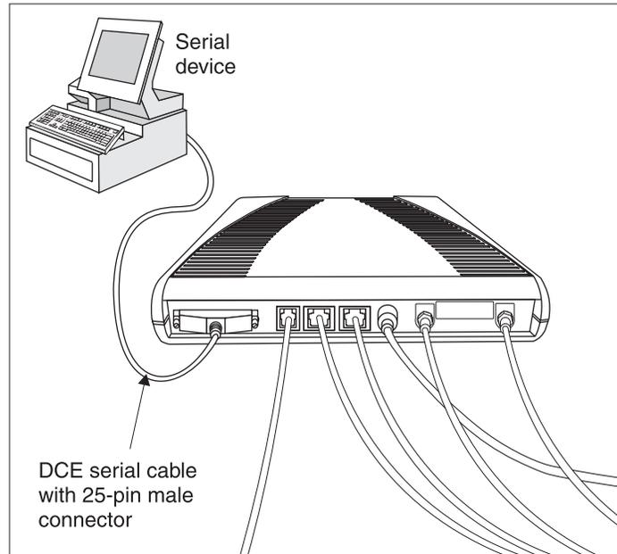
Figure 3: Connecting a serial device to the DW7700
