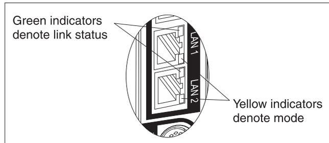
Figure 4: Dual Ethernet ports
